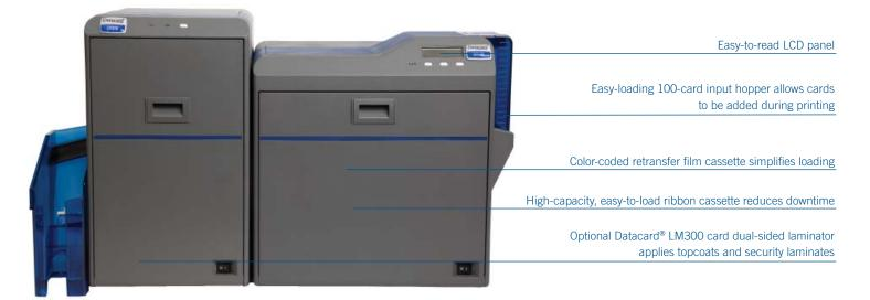
The Datacard® SR300 retransfer card printer can produce high-quality, dual-sided cards on a variety of materials.
