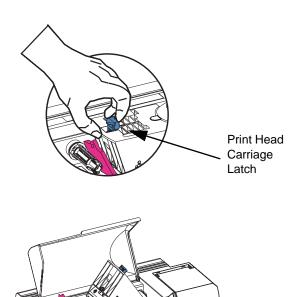
**d.** Remove the print head protection pad. Keep the pad, as well as the other packing material and the shipping carton, in case the printer is shipped or moved. If the original material is lost, a replacement Shipping Kit can be ordered from Zebra; please refer to the Media List on the Windows Drivers and User Documentation CD supplied with this printer.
