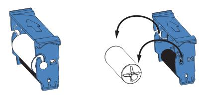
**4.** Install new cleaning roller into the Card Cleaning Cartridge. To avoid contamination, always hold the cleaning roller by the ends. (For replacement cleaning rollers, please refer to the Media List on the Windows Drivers and User Documentation CD supplied with this printer.)
