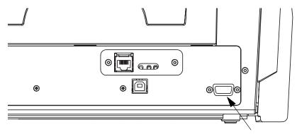
DB-9 Connector location for Smart Card Contact Station
