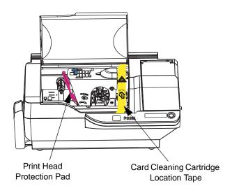
**c.** Release the Print Head Carriage by pushing the Print Head Carriage Latch to the left, and raise the Print Head Carriage. It will remain open at about a 45° angle.
