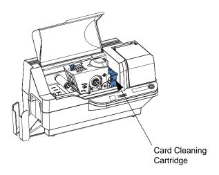
**2.** Gently remove the Card Cleaning Cartridge. Lift the "handle" end, and then pull it away from the printer.
