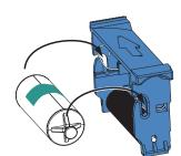
**2.** Peel the protective wrapper from the Adhesive Roller.
