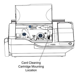
**4.** Locate the slot at the rear of the Card Cleaning Cartridge mounting location; see below.
