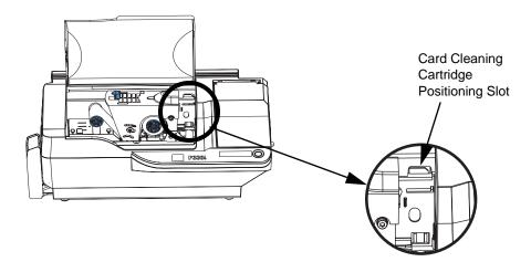
**5.** Hold the Card Cleaning Cartridge by the extended "handle" (so the large arrow on the top is pointing away from you). With the cartridge at about a 30° angle (pointing downward), insert the lip of the cartridge into the slot, until the cartridge seats against the back wall. Then press the front of the cartridge down until it seats all the way down and latches with an audible "click". See below.
