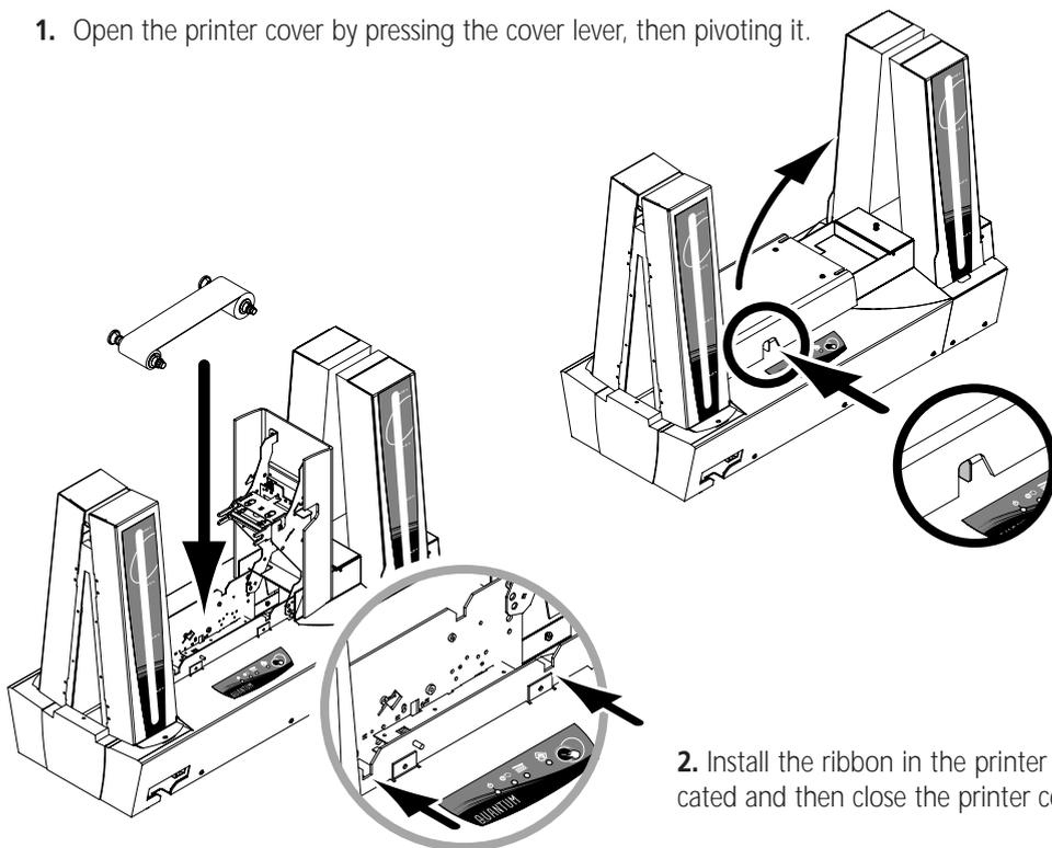
2. Install the ribbon in the printer as indicated and then close the printer cover.
