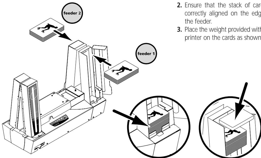
2. Ensure that the stack of cards is correctly aligned on the edge of the feeder.
