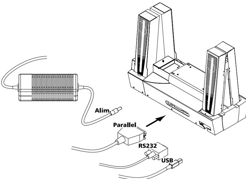
1. Connect the interface cable supplied with your printer as shown above
