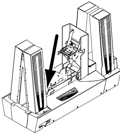
The Contact Station is a module installed in factory on Quantum Smart printers.
