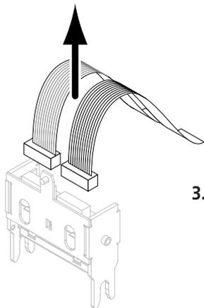
3. Disconnect the two cables located behind the print head
