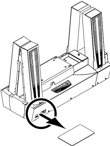
5. After a few seconds, the printer cleaning is performed and the used card is ejected into the reject box 1.
